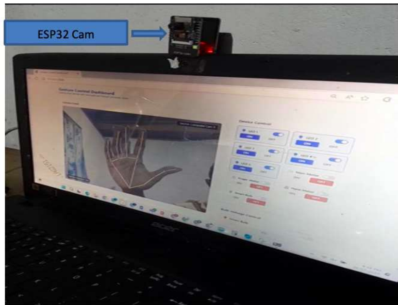
Figure 2. Hardware testing of gesture control system with ESP32-CAM and dashboard interface.
