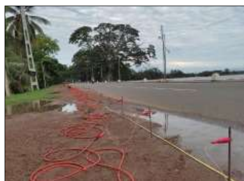
Fig. 3. Ground Electrical Resistivity Survey (GERS) at Thissa dam
